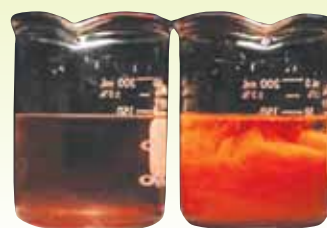
untreated yellow iron oxide in water HS treated yellow iron oxide in water
