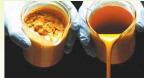
untreated yellow iron oxide in ethylhexylpalmitate
